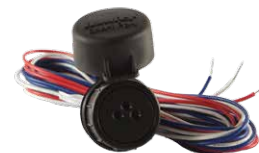
SmartPort Hunter remotes require the installation of a SmartPort wiring harness. The SmartPort is a connector that is wired to the terminals on the controller, and allows quick connection to any Hunter remote.
